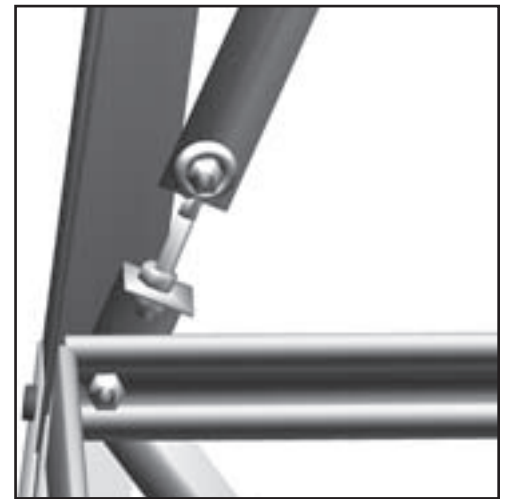
Leg Connection Backside View
